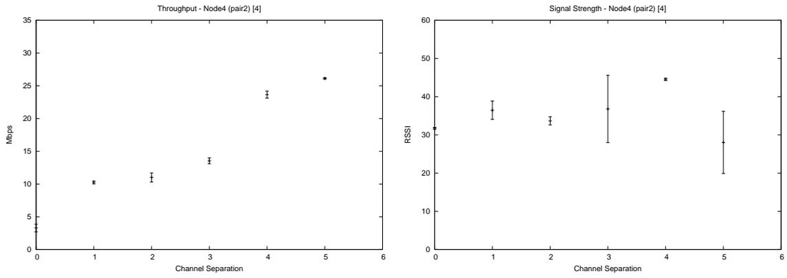
Figure 3: Signal and throughput measurements, throughput increases steadily but is poor on channel 1
