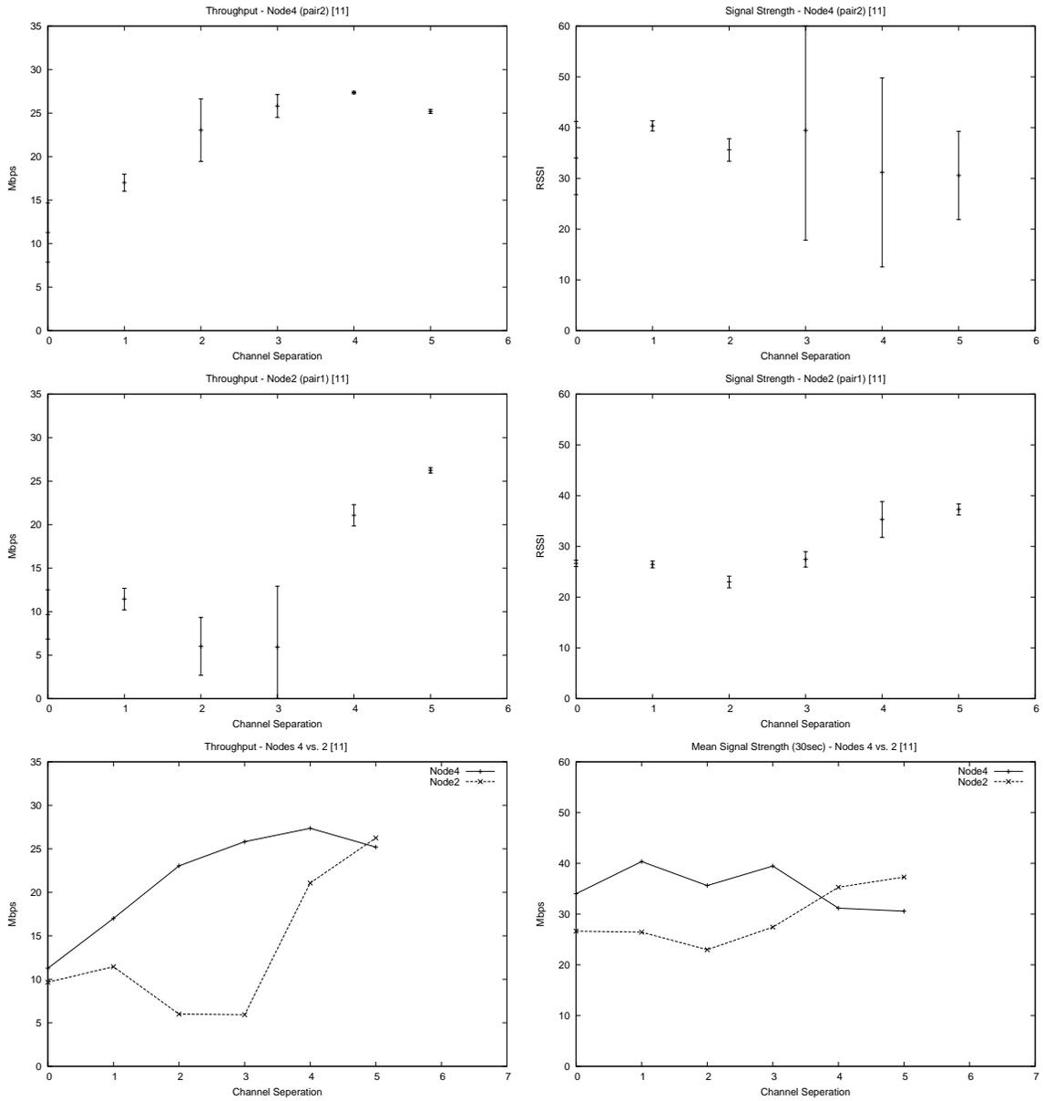
Figure 10: Signal and throughput measurements from each network, and overlapping comparisons. Height separated, outside interference - additional interference from cars.
