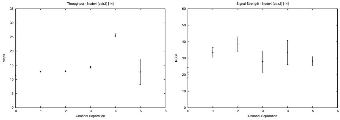
Figure 13: Signal and throughput measurements, no improvement in routing height-separated case
