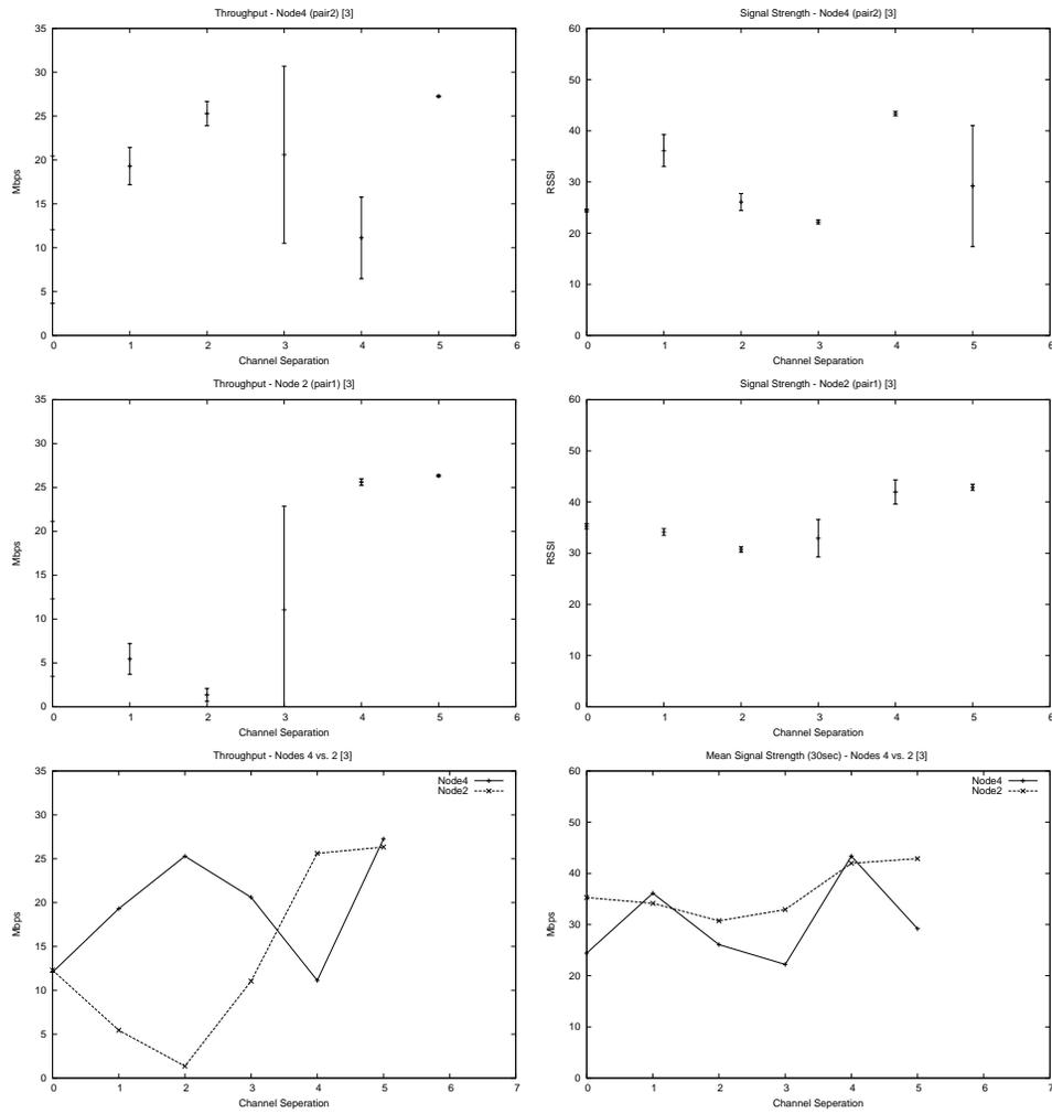
Figure 2: Signal and throughput measurements from each network, and overlapping comparisons. Notice how the throughputs are almost mirror images of each other. In this case pair2 dominated the spectrum
