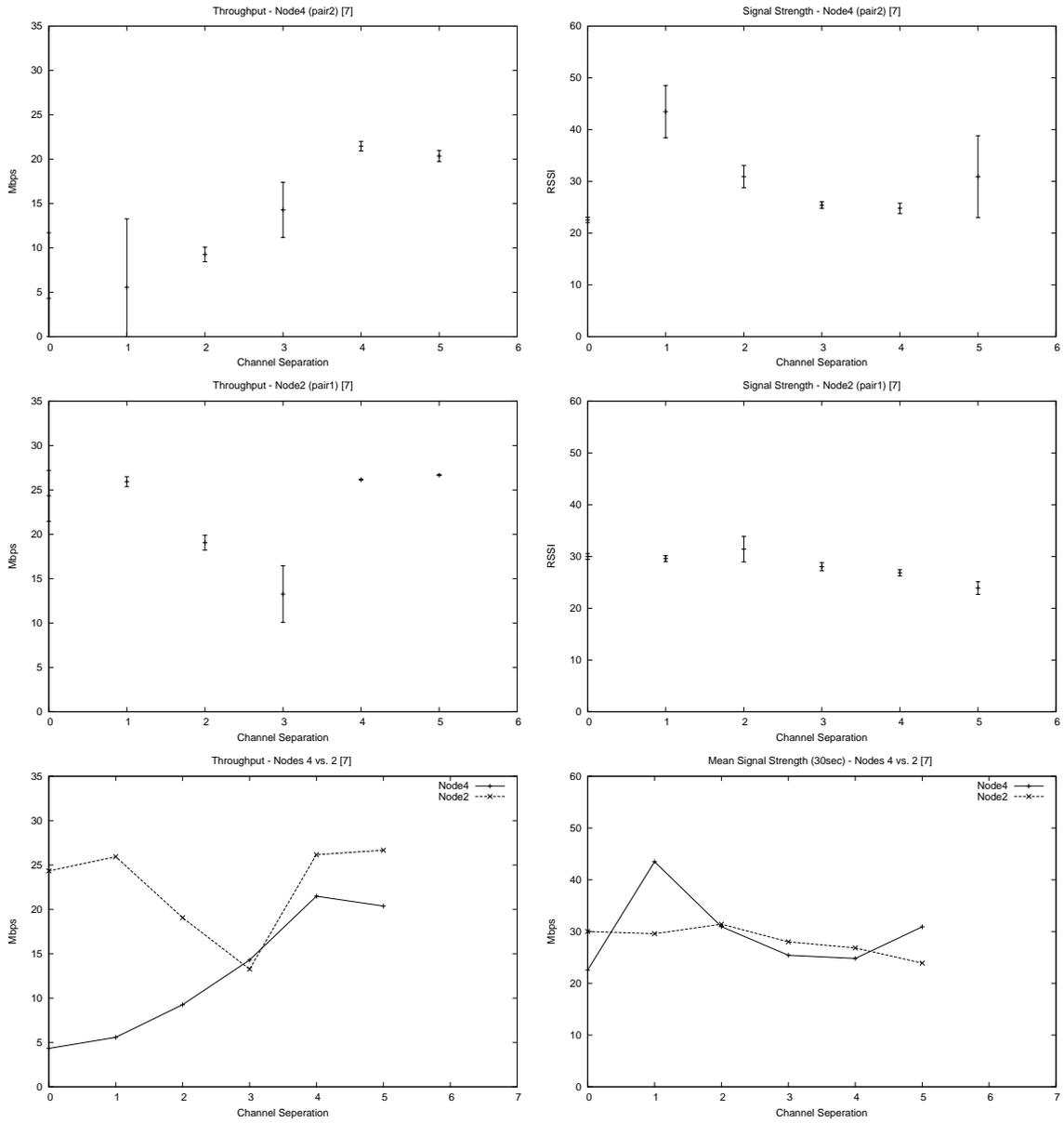
Figure 6: Signal and throughput measurements from each network, and overlapping comparisons. 90° configuration, pair1 network is dominating the available bandwidth on contended channels
