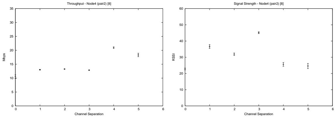
Figure 7: Signal and throughput measurements, 90 ° configuration with routing.
