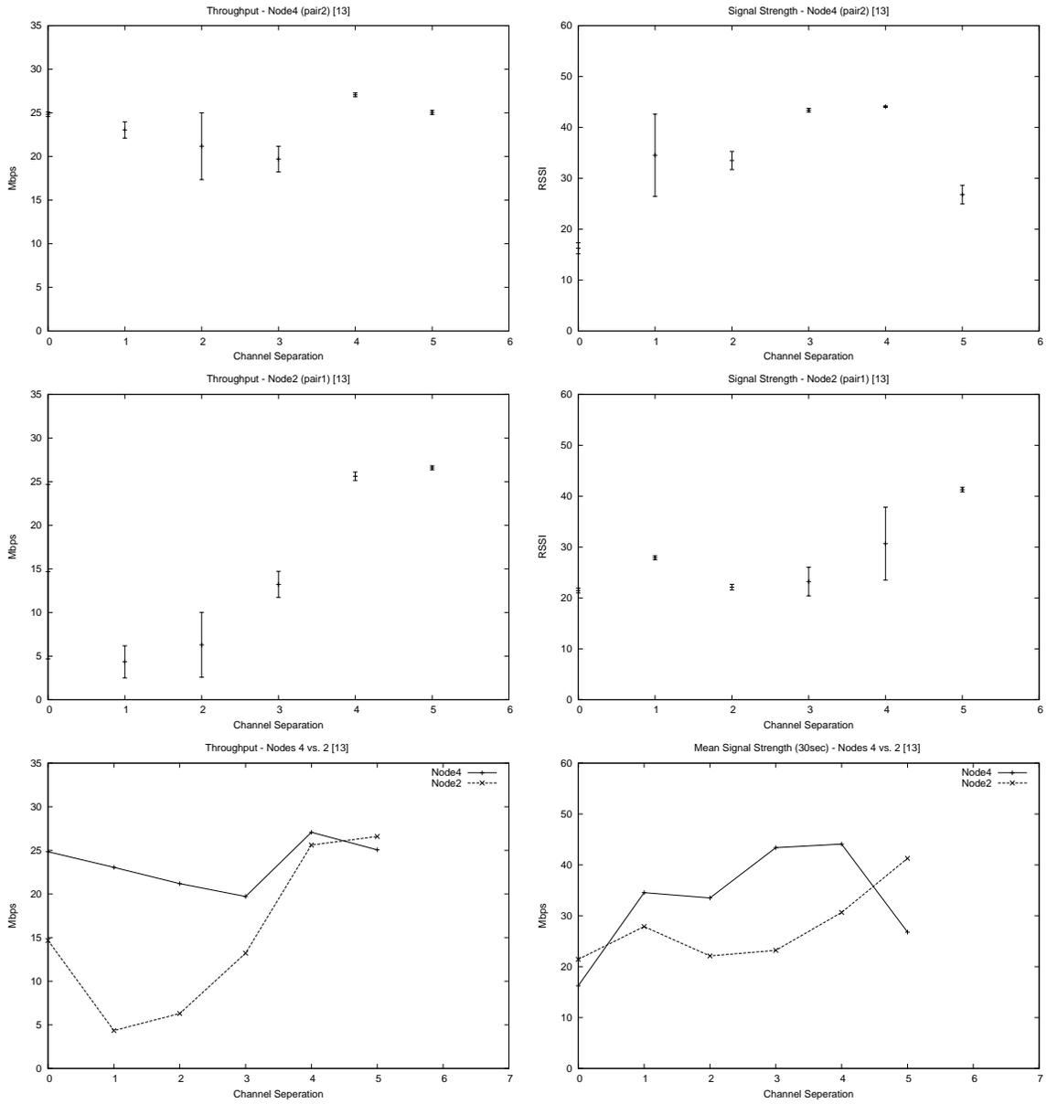
Figure 12: Signal and throughput measurements from each network, and overlapping comparisons. Height separation seems to benefit throughput.
